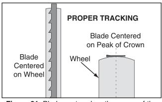
Figure 21. Blade centered on the crown of the wheel.
